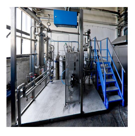
Experimental facility for studing pressurised fluidised oxy-fuel combustion and gasification of coal (1,6 MPa, 900°C, 2kg/h)
