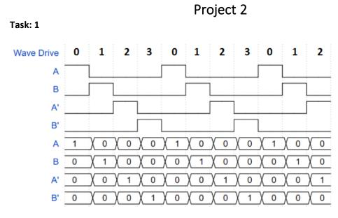
Based on waveform the following look-up table can be prepared for **Wave Drive**. Input is program counter.
