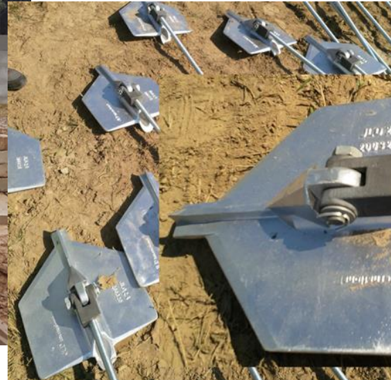
Additional steel anchors used in testing
