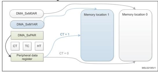
Figure 6. Double-buffer mode
