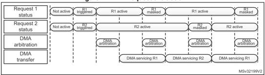
Figure 14. DMA request arbitration
