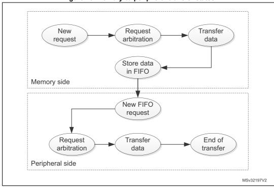
Figure 13. Memory-to-peripheral transfer states
