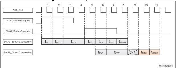
Figure 16. SPI full duplex DMA transfer time
