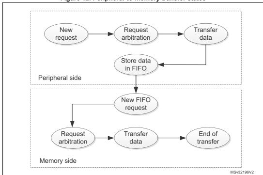
Figure 12. Peripheral-to-memory transfer states
