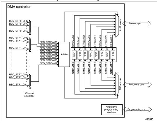
Figure 1. DMA block diagram
