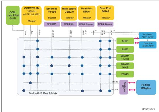
Figure 7. STM32F405/415 and STM32F407/417 system architecture
