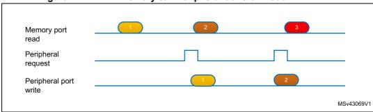
Figure 17. DMA in Memory-to-Pheripheral transfer mode
