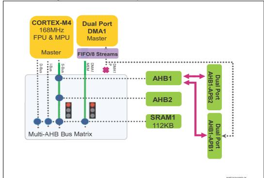
Figure 8. CPU and DMA1 request an access to SRAM1
