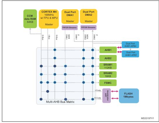
Figure 11. DMA dual port
