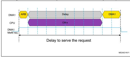
Figure 10. DMA transfer delay due to CPU transfer issued by interrupt
