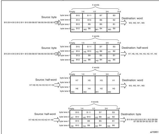
Figure 4. FIFO structure
