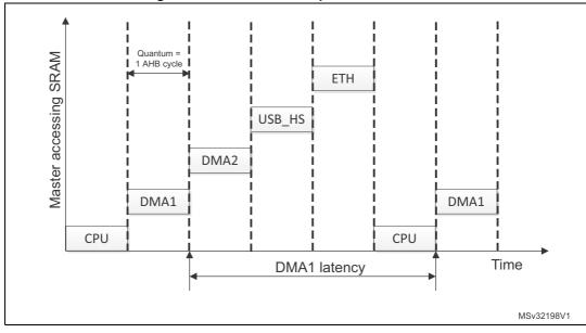
Figure 9. Five masters request SRAM access
